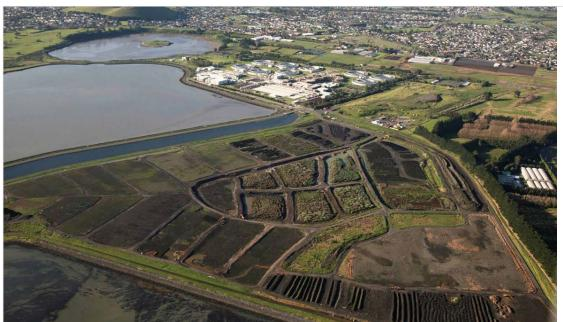
In the foreground, Pond 2, a 44 hectare area of former seabed that contains oxidation pond sludge. Pond 2 is divided into a series of cells, where biosolids are placed in layers of approximately 600 to 800 millimetres deep.
