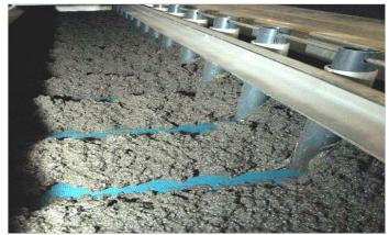
The gravity belt with thickened blended sludge.
